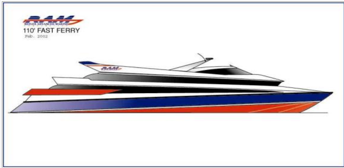
Side view of Reflex Advanced Marine's concept for a 33-metre passenger ferry built on the triple hull.
